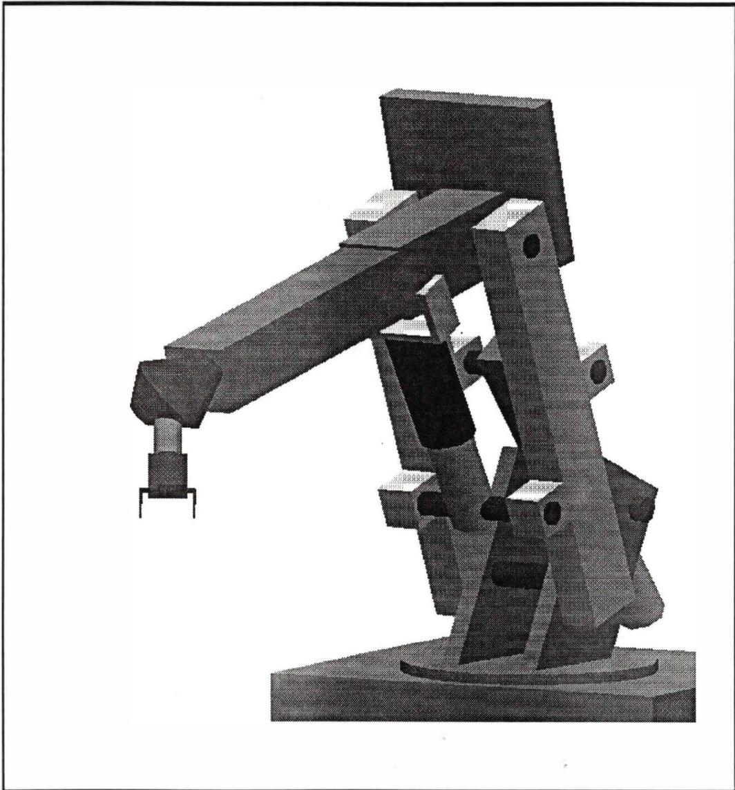
Figure 1.4 A common industrial robot often used for welding.
